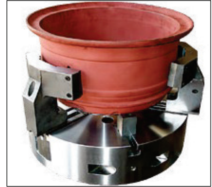
■ Special dual pressure chuck with floating jaws
